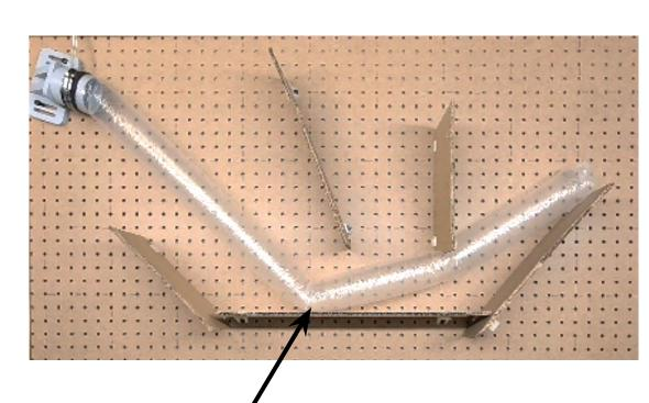
Notice how inflated tubes tend to buckle rather than curve. Rigid segments cause the body to push off inside wall
